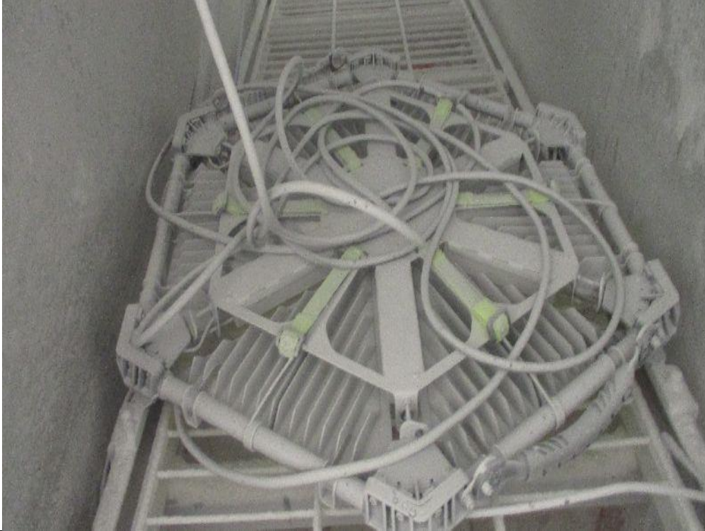
Bild / Picture 12: After dust test
