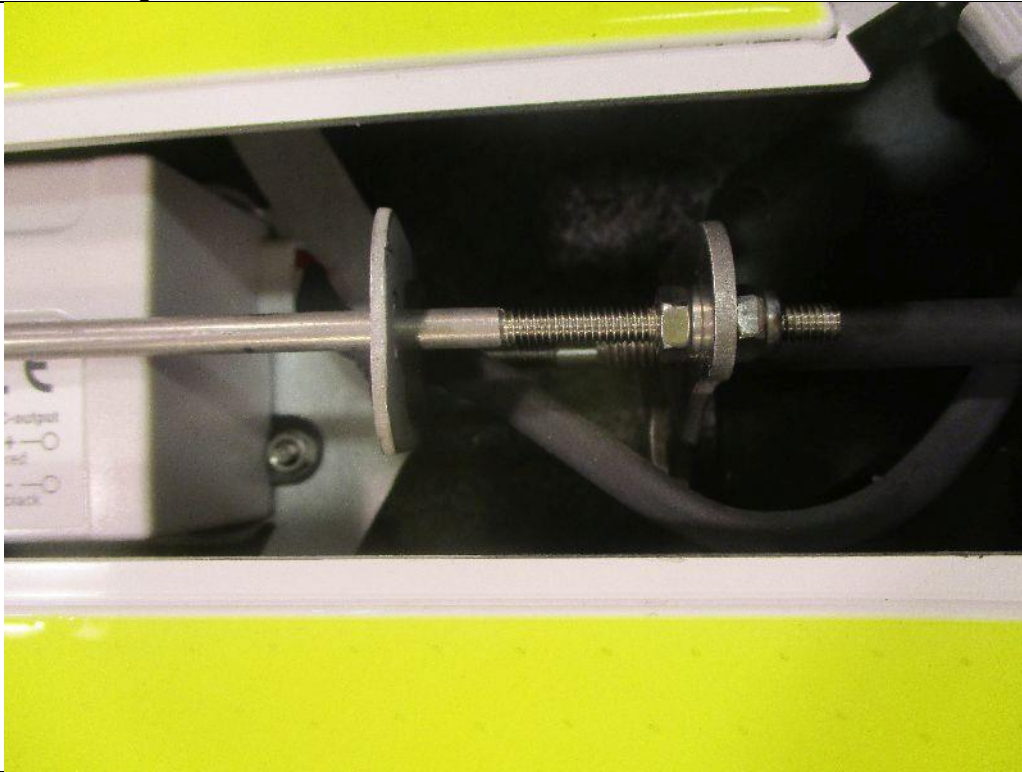
Bild / Picture 8: Securing of LED converter
